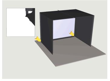
Step 41 Attach the bottom Material Clips to the Frame.
