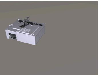
Step 50 Place the Projector Mount onto the Projector.
